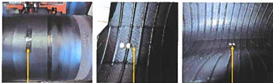
Picture 12. RFID rubber patch applied during building stage of the tire. RFID rubber patch after curing. Process is as follow: takeoff release liner, apply rubber patch on green rubber (in this case chip facing up), into the mold (high pressure, temperature around 190 degrees celsius)
