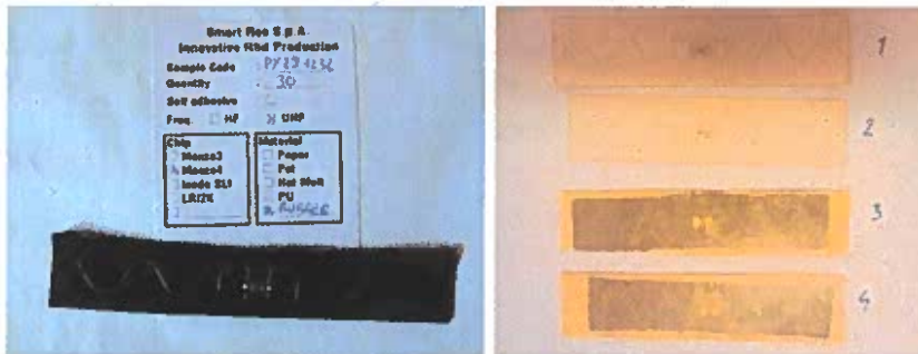
Picture 11. Rubber patch material containing liner, chip/antenna, this case rubber including. The rubber patch, one layer (without facelayer) can withstand cold vulcanization process having a temperature up till 110 degrees celsius
