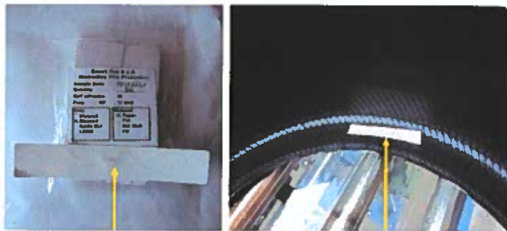
Picture 13. One release liner, RFID chip/antenna, pressure sensitive, heat activating adhesive, face layer melting point greater than 170 degrees Celsius, non-woven, single layer, face layer is cotton paper. Right picture cotton paper RFID label applied on a "green" unvulcanized tire
